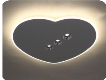
PRD-C 0969L-C 26Wx2 3000K 4000K MODE:2.4G remote control Material:iron+acrylic LED:CRI 80 75-95LM/W Size:495x465x38 Color:WH FR
